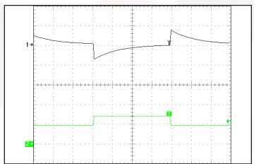
Figure 11: Output voltage response to step-change in load current (50%-75%-50% of lout(max);  $dI/dt = 0.1 \ A/\mu sec$ ). Output capacitance:  $100\mu F$  electrolytic in parallel with  $1\mu F$  ceramic. Ch 1: Vout (5V/div), Ch 2: lout (2A/div). Horizontal Scale: 100msec/div
