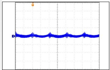
Figure 10: Output voltage ripple at nominal input voltage and rated load current. Output capacitance:  $100\mu F$  electrolytic in parallel with  $1\mu F$  ceramic. Ch1: Vout (200 mV/div, BW= 20MHz). Horizontal Scale:  $2\mu sec/div$ .
