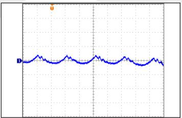
Figure 9: Input terminal current ripple at full load and nominal input voltage. Output capacitance:  $100\mu F$  electrolytic in parallel with  $1\mu F$  ceramic. Ch 1: Input (1.0A/div, BW=20MHz). Horizontal Scale:  $2\mu sec/div$ .
