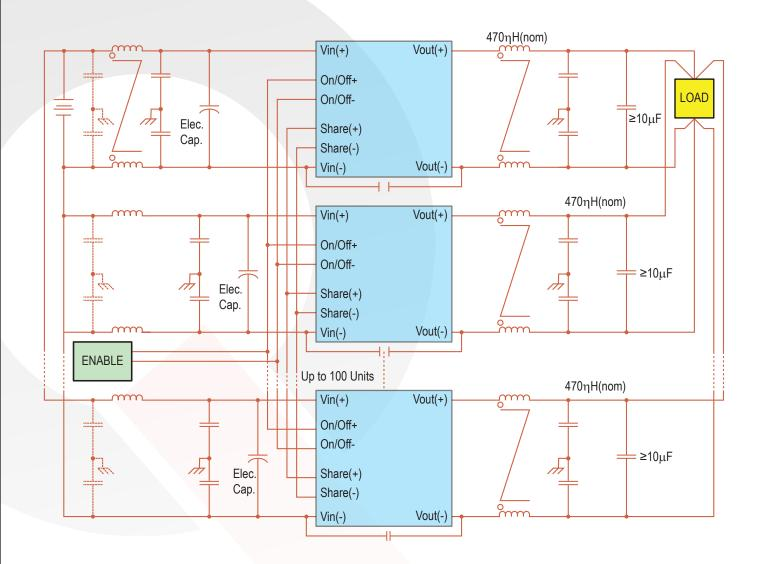
Figure F: Typical Application Circuit for Paralleling of Full-Featured Units with an Input Common-Mode Choke. If an input common-mode choke is used, Vin(-) may be tied together either before or after the choke for each unit. 470 nH (nominal) inductor or an output common-mode choke is required. See Figure G for output common-mode choke configuration.
