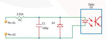
Figure B: Internal ON/OFF Pin Circuitry
