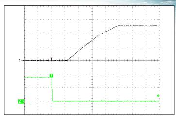
Figure 8: Typical startup waverform with 100% load and 680µF output capacitance. Input voltage pre-applied. Ch 1: Vout (100V/div). Ch2: ON/OFF Pin(10V/div). Horizontal Scale: 100msec/div
