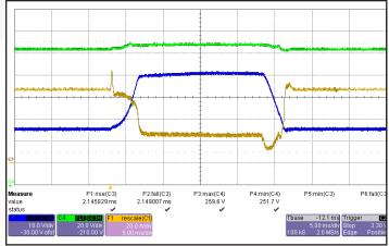
Figure 12: Output voltage response to step-change in input voltage (16V-40V-16V; 10V/ms,  $100 \mu F$  output capacitor). Ch 3: Vin (10V/div), Ch 4: Vout (20V/div), Ch F1: Iin (20A/div).
