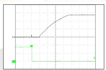
Figure 7: Typical startup waveform with 0% load and 680µF output capacitance. Input voltage pre-applied. Ch 1: Vout (100V/div). Ch2: ON/OFF Pin (10V/div). Horizontal Scale: 100msec/div
